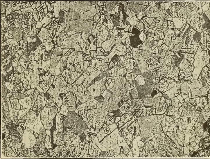
FIG. 7.—Longitudinal section of copper cylinder annealed at 650° C. \times 100
